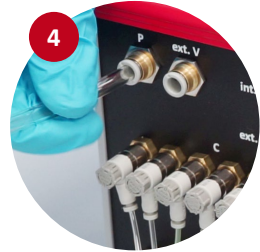
Connect the tube to [3] compressed air connection labeled with "P"
