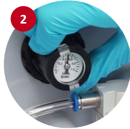
Set air pressure outlet to 5-6 bar (outlet closed)
