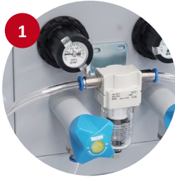
Connect air pressure outlet with air filter
